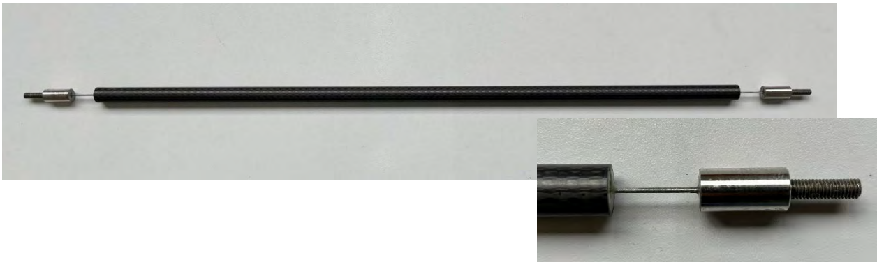
Figure 18: Example of designed stinger – stiff tube (CFRP) and joint like end sections (steel)
