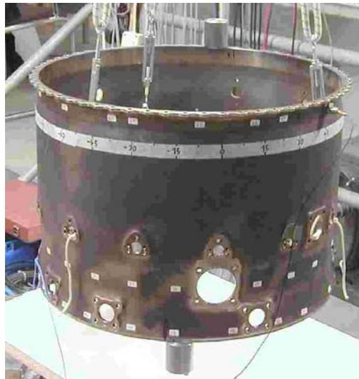
Figure 2: CCOC with tuning masses attached to the flanges for modal survey test
