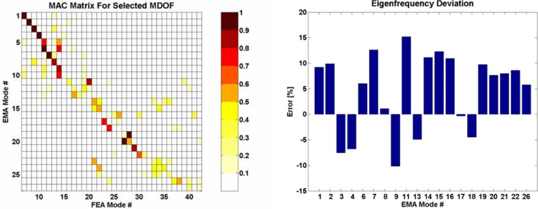
Figure 3: Correlation results of test data and analytical data of the initial model after remodeling
