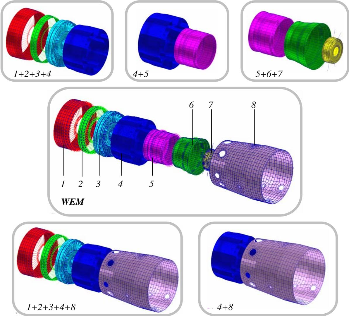
Figure 7: Exploded view on whole engine model and different subassembly models
