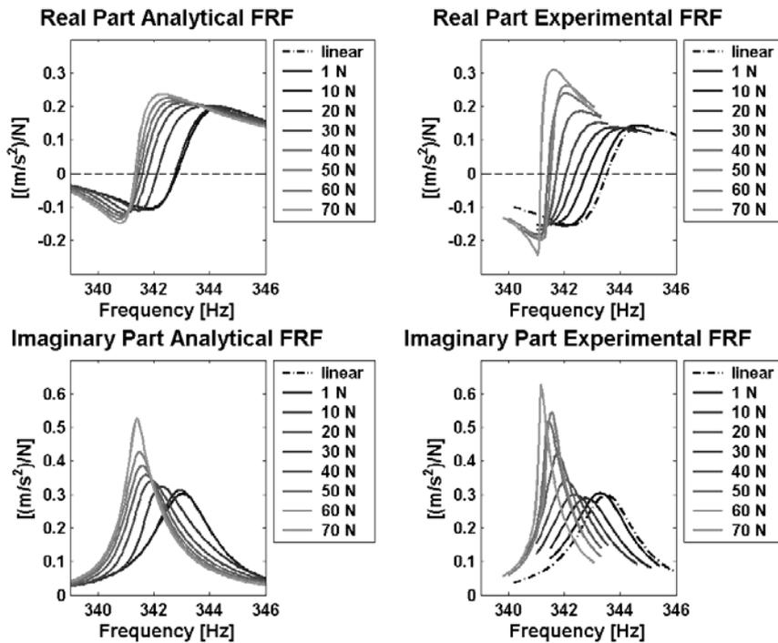
Figure 13: Comparison of analytical and experimental non-linear FRFs for different excitation force levels after non-linear updating
