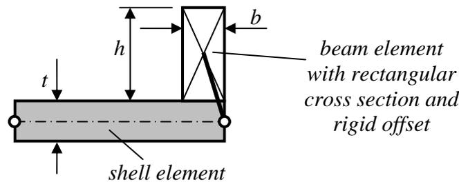
Figure 4: Beam element eccentrically connected to a shell element node by a rigid offset
