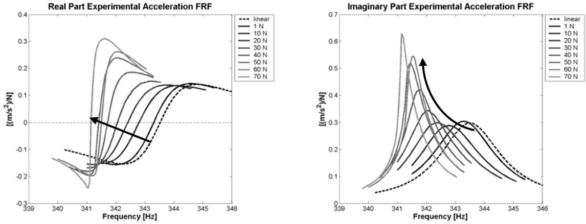
Figure 10: Non-linear experimental FRFs measured at the driving point
