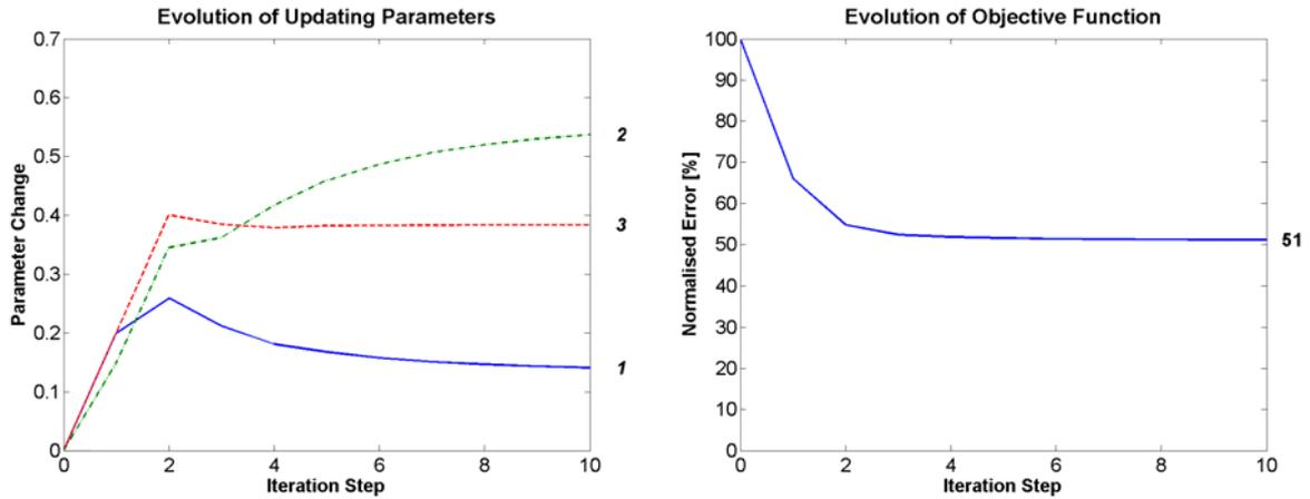
Figure 12: Evolution of non-linear updating parameters and normalized objective function
