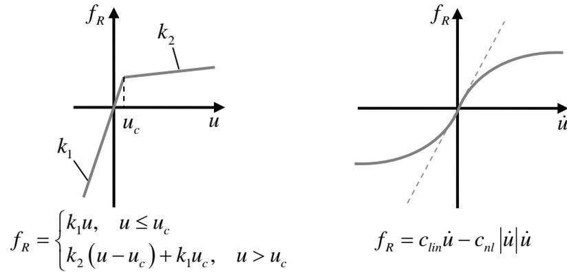
Figure 11: Restoring force of bilinear spring and softening quadratic damper
