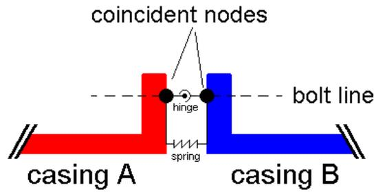
Figure 8: Principle arrangement for joint modeling
