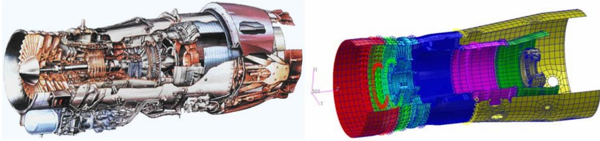
Figure 1: Aero-engine with accessories and WEM w/o accessories (ca. 105.000 degrees of freedom)
