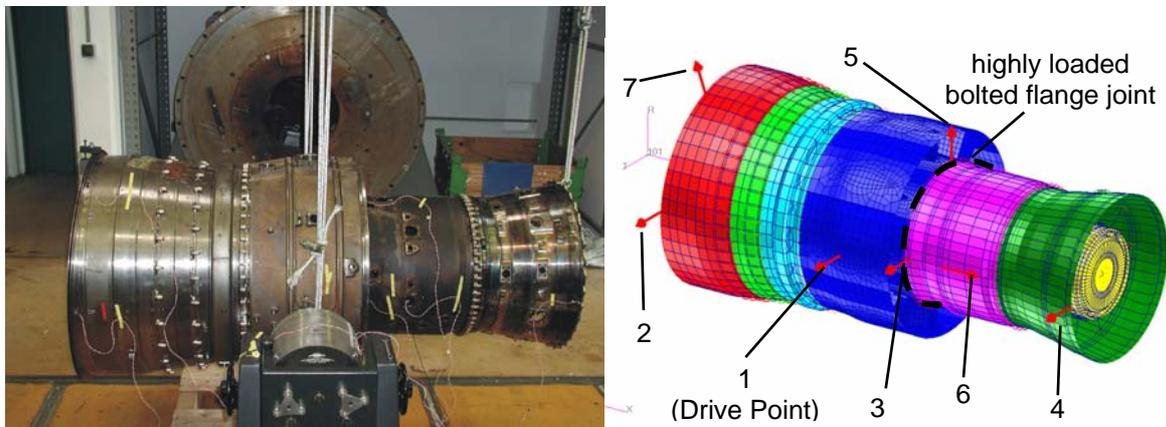
Figure 9: Test setup for non-linear step-sine tests and FE model with measurement positions
