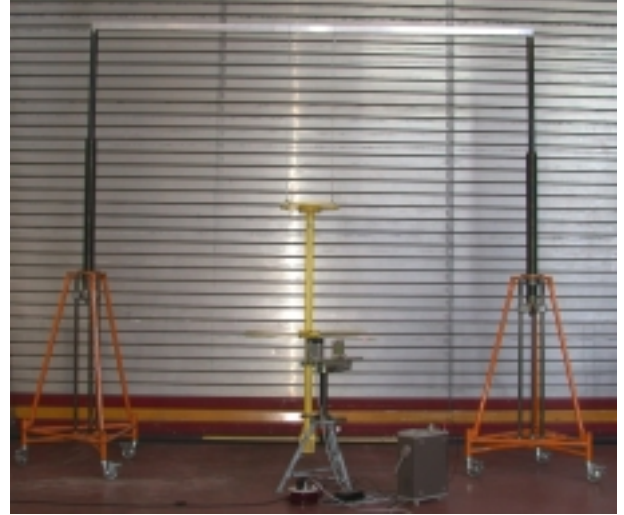
Figure 4: Measurement of moments of inertia for Clumod with four blades
